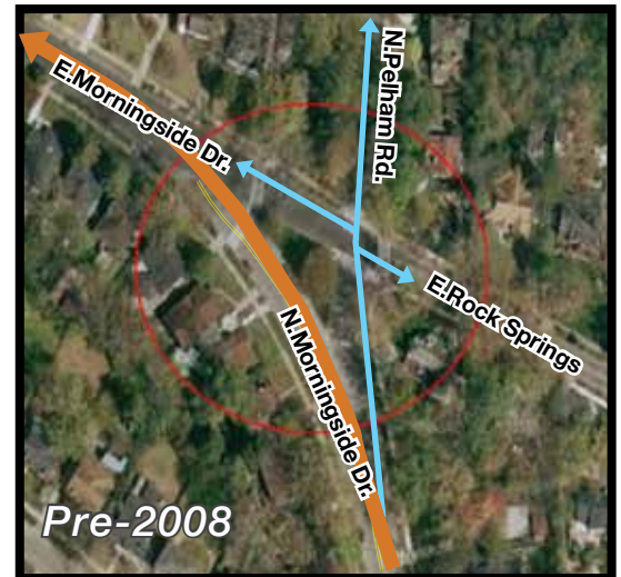
Prior to 2008: The majority of northbound traffic through the Morningside/Rock Springs intersection is directed onto E. Morningside Dr. Image via atlantaga.gov.
