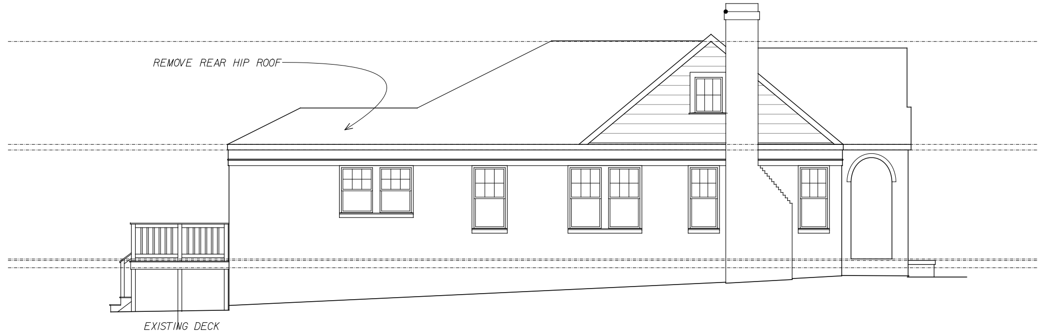
01 EXISTING LEFT SIDE ELEVATION A-1.04 SCALE: 1/8" = 1'-0"
